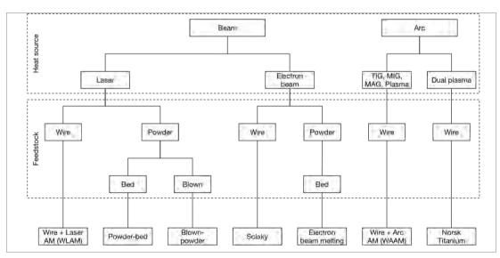
Figure 1: Comparison of additive manufacturing processes (Marinelli et al, 2017, first published in Bulletin #173)
