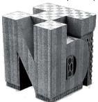
LBM printed with AMtrinsic® Ti-42Nb powder & Niobium GmbH)
