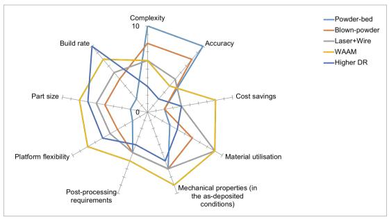
Figure 2: Comparison of additive manufacturing processes (Marinelli et al, 2017)
